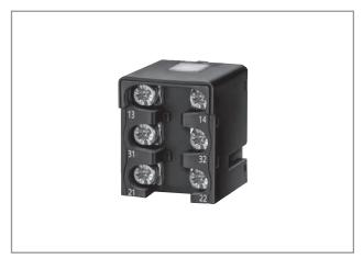
The three-pole switching block (2 NC, 1 NO) in snap-action and slow-action is regularly available for all enclosure forms. It offers more switching through redundant shutdowns (2 NC contacts) with simultaneous signaling (1 NO contact). The same installation space is required as for a two-pole switching block.
