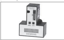
The Ammeter Display Units plug into the Sensitrip Trip Unit and displays the phase current flowing in the breaker. They are powered by the breaker's CT's with replaceable battery back-up for maintaining trip and max logs.
