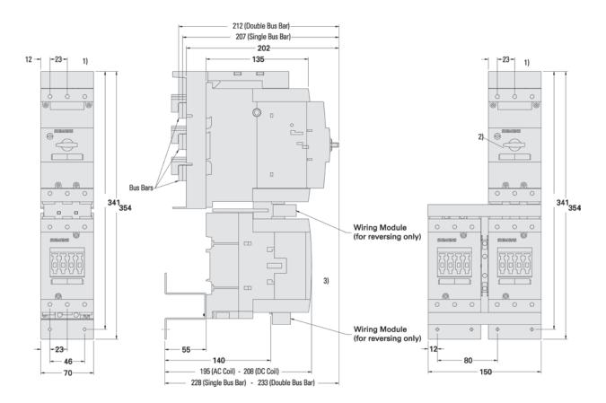
Lateral clearance to grounded components minimum 6 mm.
