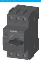
SIRIUS 3RV Motor Starter Protectors (MSPs) are built for a wide range of applications and meet the requirements of control users worldwide. Each MSP features a manual ON/OFF switch, a Class 10 adjustable bimetallic overload relay (Class 20 available in the two largest frame sizes), and magnetic trip elements for short circuit protection.
