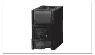
The current measuring modules are designed as system components for connecting to evaluation units 3RB22 to 3RB24. Using these evaluation units the motor current is measured and the measured value sent to the evaluation unit for evaluation. The current measuring modules in sizes S00 to S3 up to 55 mm wide are equipped with straight-through transformers and can be snap-fitted under the evaluation units. The larger evaluation units are installed directly on the contactor or as stand-alond units.
